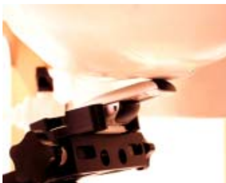
Figure 8.5 Left Head SAR Test Setup -- Ear/Tilt 15° Position--
