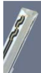
Figure 3.4 Probe Thick-Film Technique
