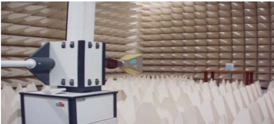
Figure2. Photograph of 3m Fully Anechoic Chamber
