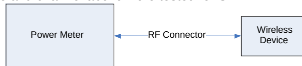
Figure 9-3 Power Measurement Setup
