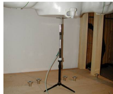
Figure 10-2 System Verification Setup Photo
