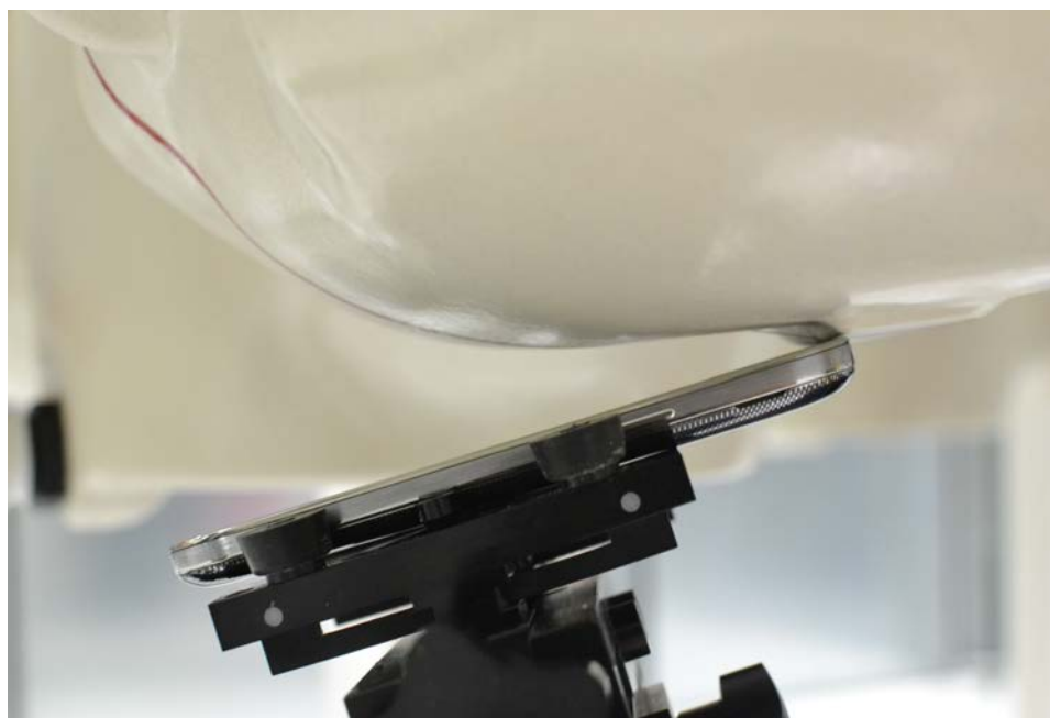
SAR Test Setup Photo 4: Left Tilt
