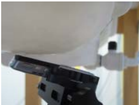
Figure 8.3 Right Head SAR Test Setup -- Ear/Tilt 15° Position--
