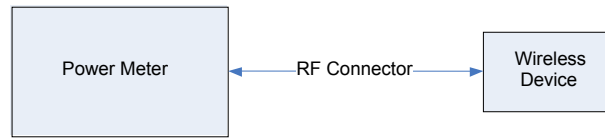
Figure 9-3 Power Measurement Setup
