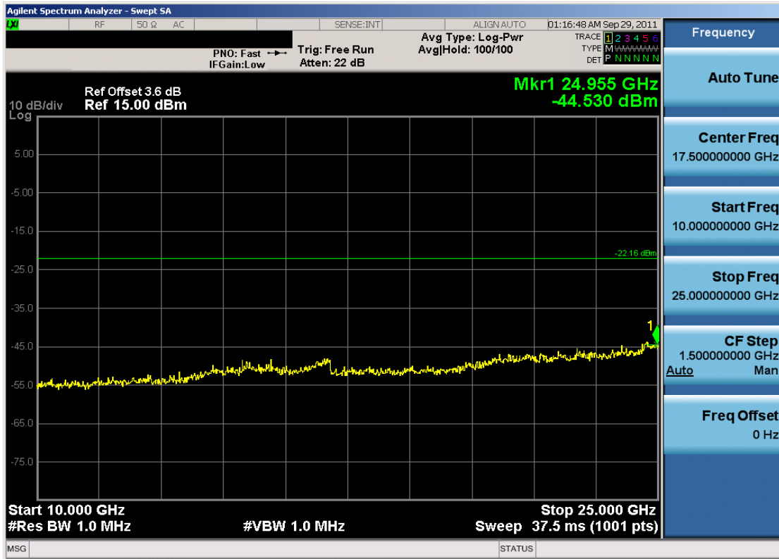
Plot 6-26. Conducted Spurious Plot (802.11b - Ch. 1)
