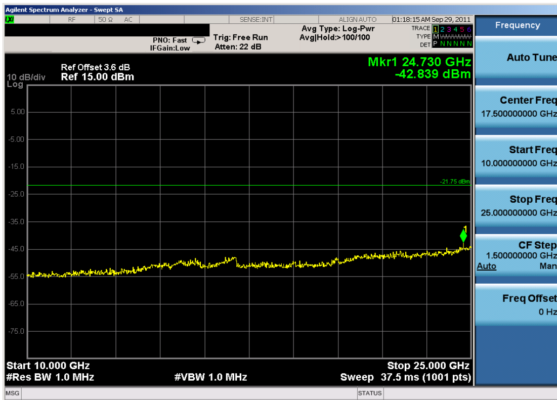
Plot 6-28. Conducted Spurious Plot (802.11b – Ch. 6)
