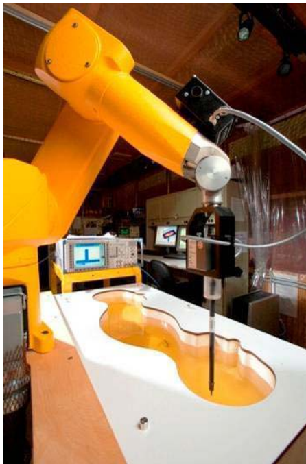
Figure 3-2 DASY4 SAR Measurement System
