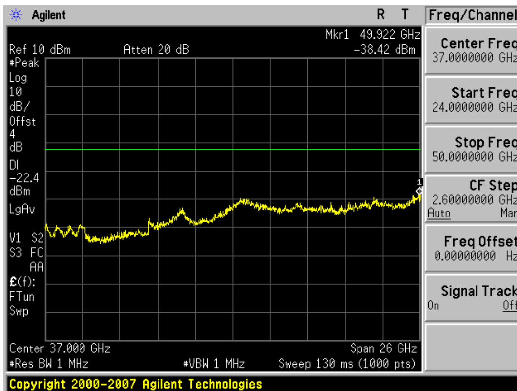
Plot 6-48. Conducted Spurious Plot (802.11a – Ch. 149)
