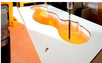
Figure 6-2 SAM Phantom with Simulating Tissue
