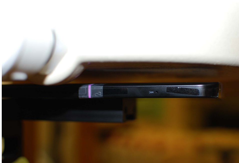
Figure 20-2 SAR Test Setup Photo 2- Back Side at 1.0 cm (without power back-off)
