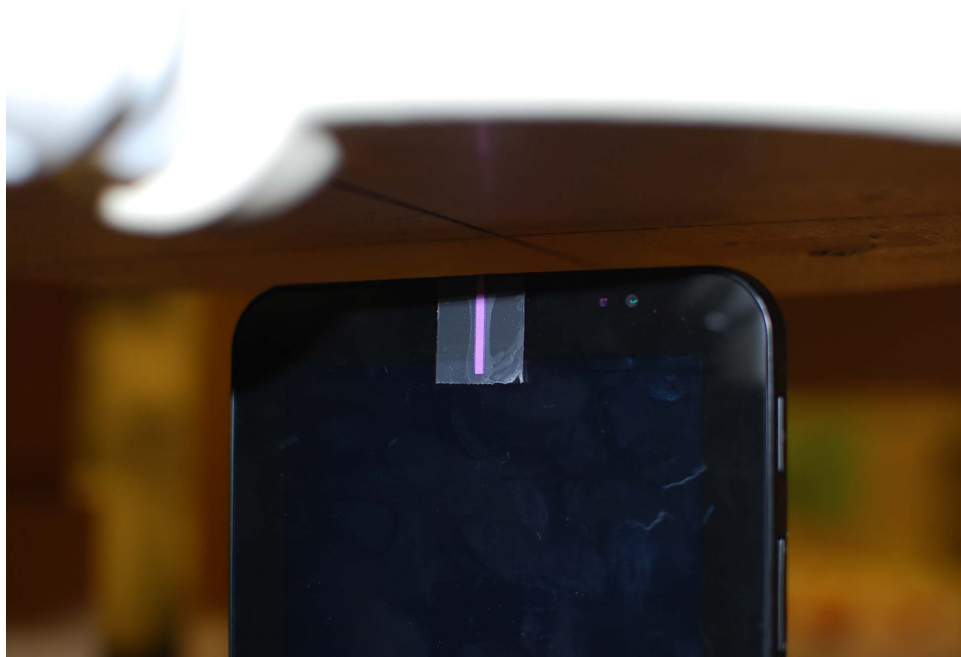
Figure 20-3 SAR Test Setup Photo 2 - Top at 0.5 cm
