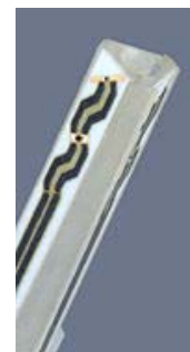
Figure 3.4 Probe Thick-Film Technique
