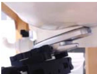
Figure 8.9 Left Head SAR Test Setup -- Ear/Tilt 15° Position--
