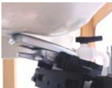
Figure 8.3 Right Head SAR Test Setup -- Ear/Tilt 15° Position--
