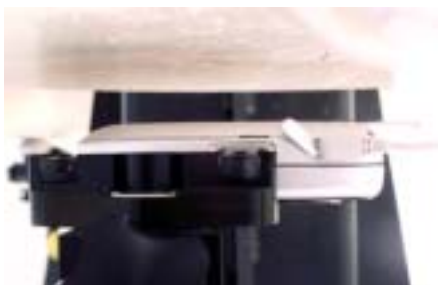
Figure 8.10 Body SAR Test Setup -- w/o Holster--
