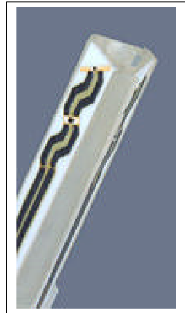
Inside view of ET3DV6 E-field Probe
