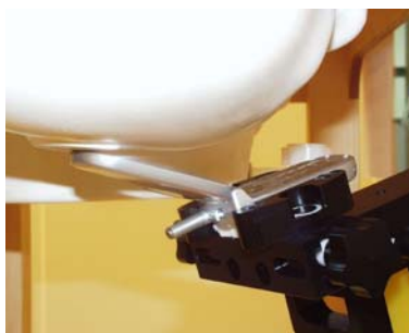
Figure 8.5 Right Head SAR Test Setup -- Ear/Tilt 15° Position--
