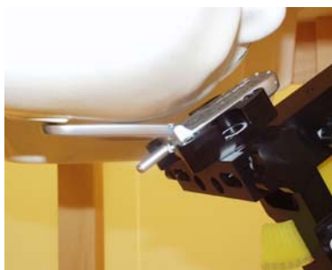
Figure 8.4 Right Head SAR Test Setup -- Cheek / Touch Position--
