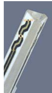
Figure 3.4 Probe Thick-Film Technique
