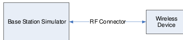
Figure 12-1 Power Measurement Setup
