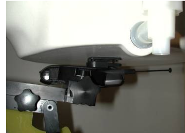
Figure 9-4 Body SAR Sample Photo (Not Actual EUT)
