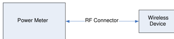
Figure 12-2 Power Measurement Setup
