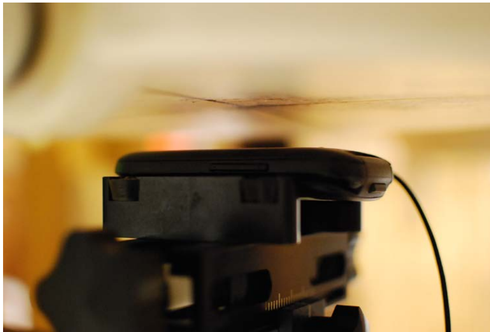
SAR Test Setup Photo 4 – Body-Worn at 1.5 cm
