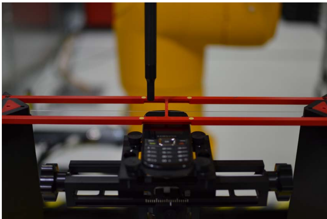
Figure 18-1 Ear Reference Point HAC Phantom Alignment
