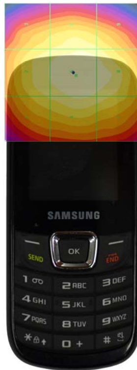
Figure 18-4 E-Field WD Scan overlay
