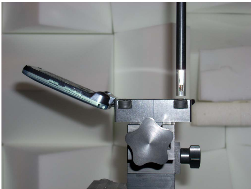
Figure 12-2 Test Setup for Wireless Device
