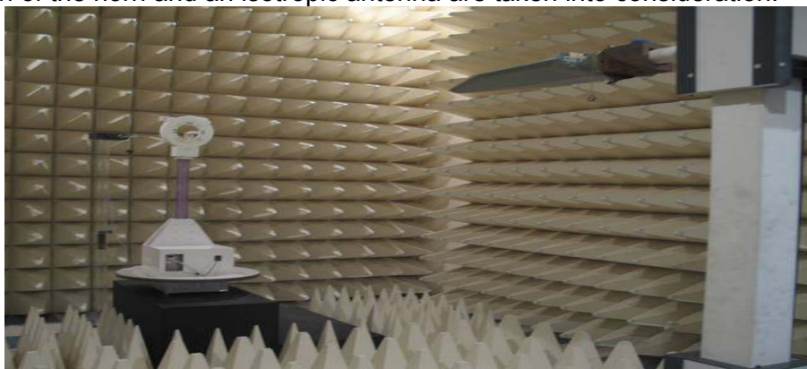
Figure2. Photograph of 3m Fully-Anechoic Chamber
