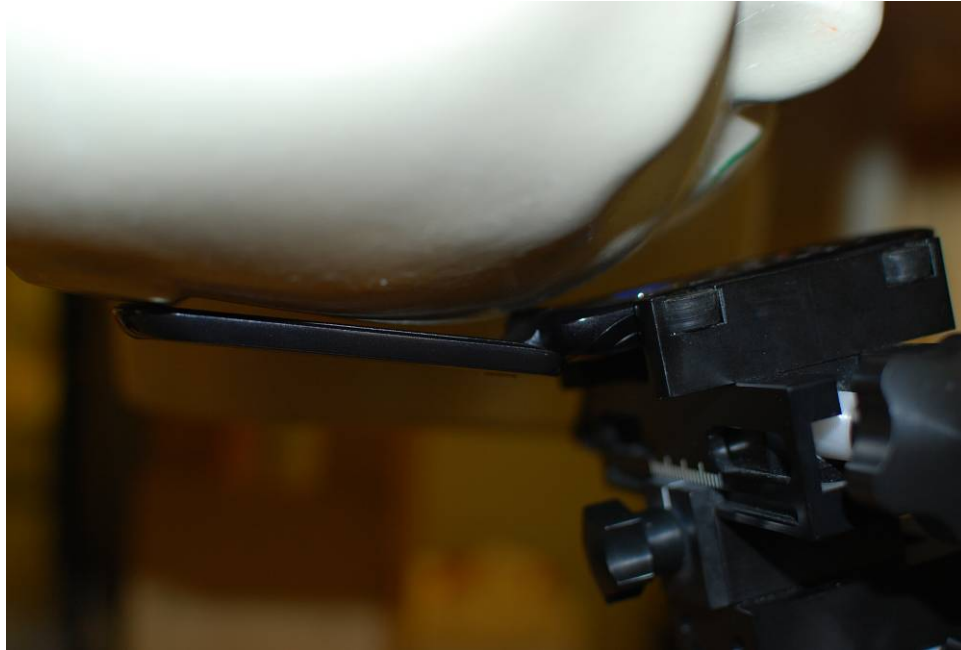
Figure 19-1 SAR Test Setup Photo 1 – Right Touch
