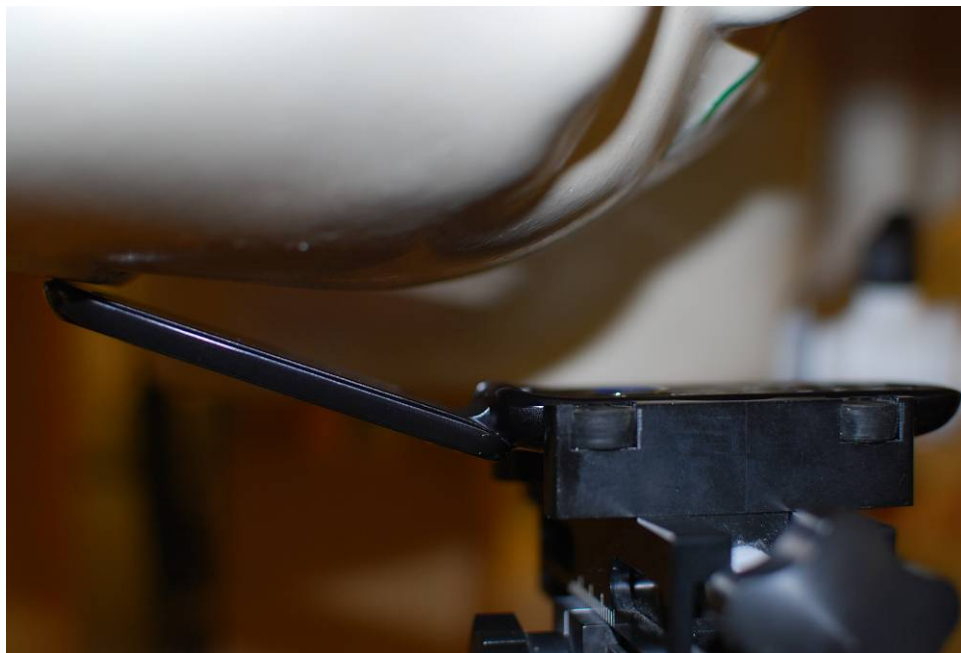
Figure 19-2 SAR Test Setup Photo 2 – Right Tilt
