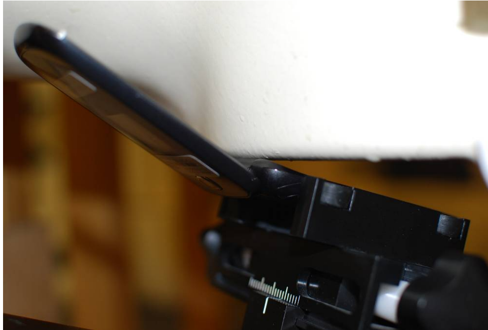
Figure 19-5 SAR Test Setup Photo 5 – Mouth/Jaw
