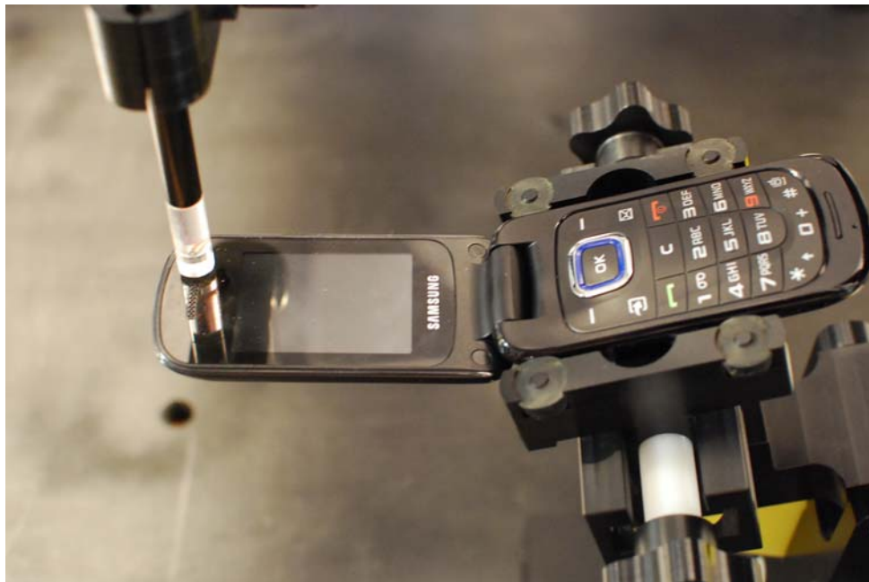
Figure 13-2 Test Setup for Wireless Device
