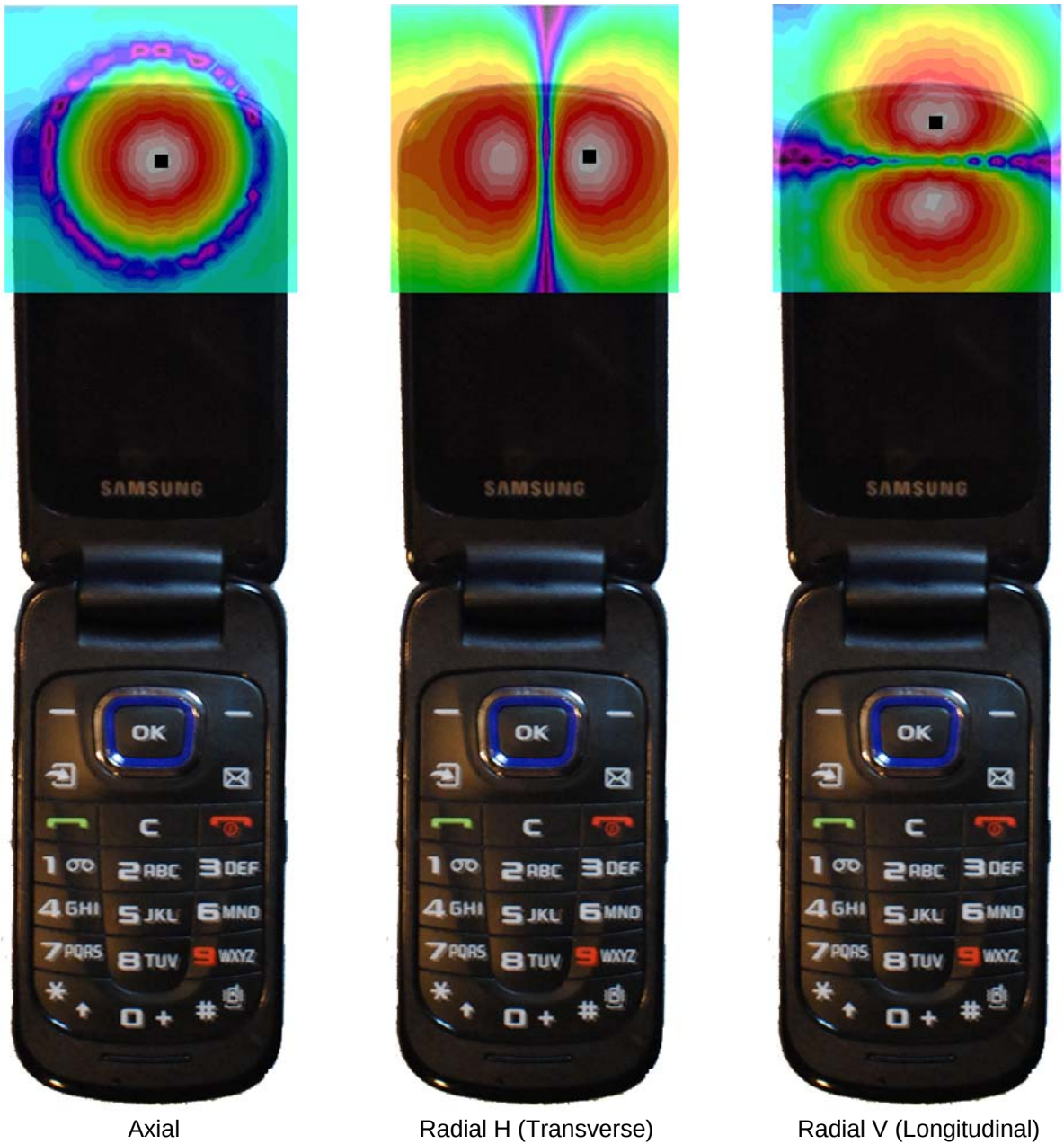
Figure 13-3 T-Coil Scan Overlay Magnetic Field Distributions
