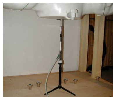
Figure 12-2 System Verification Setup Photo
