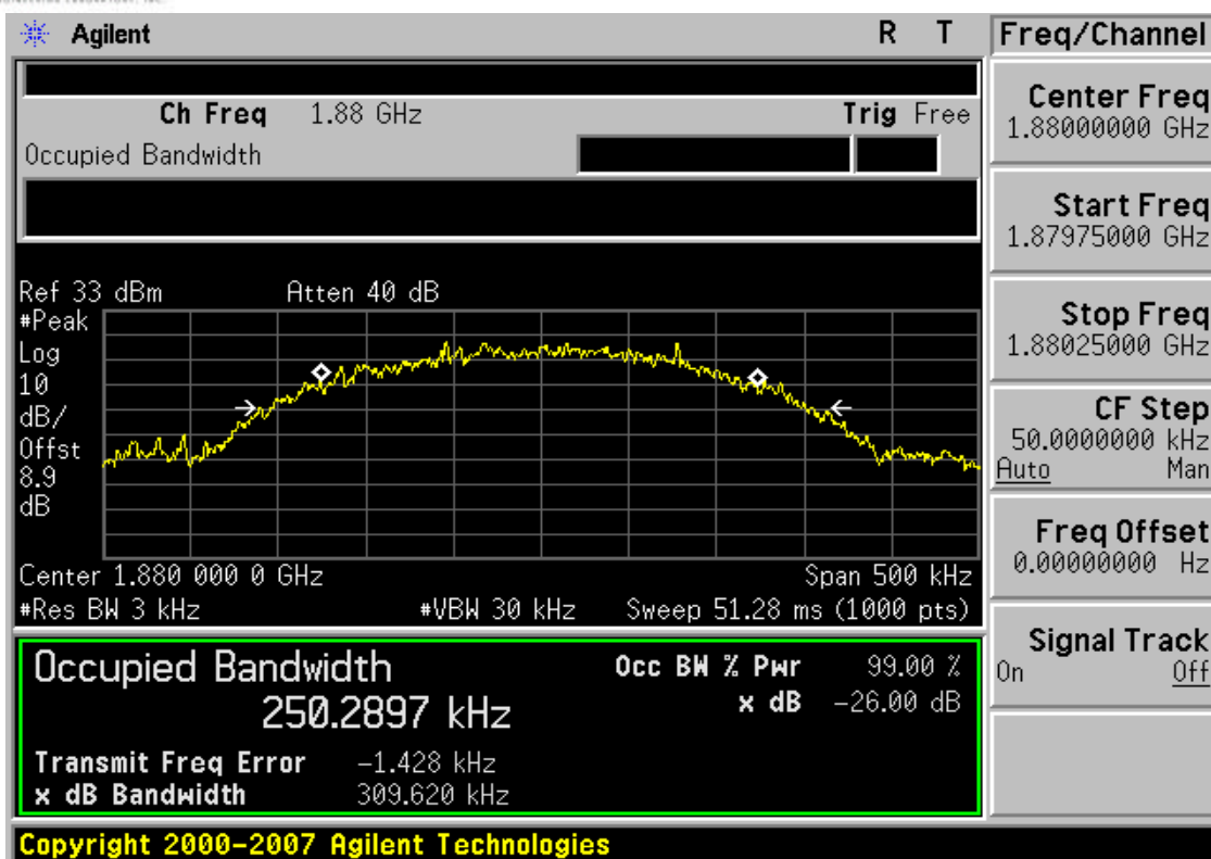
Plot 7-21. Occupied Bandwidth Plot (EDGE1900 Mode – Ch. 661)
