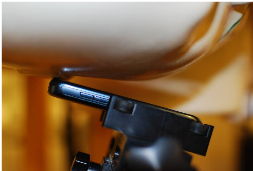
Figure 20-2 SAR Test Setup Photo 2
