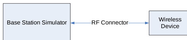
Figure 11-1 Power Measurement Setup
