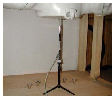
Figure 14-2 System Verification Setup Photo
