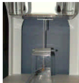
Figure A-1 Dipole Validation Test Setup
