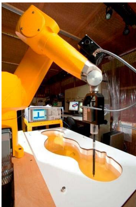
Figure 3-2 DASY4 SAR Measurement System
