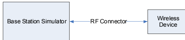
Figure 13-1 Power Measurement Setup
