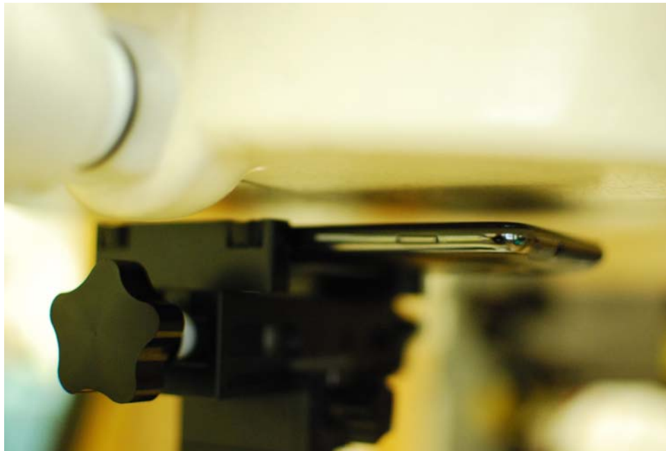
SAR Test Setup Photo 6: Front at 1.0 cm
