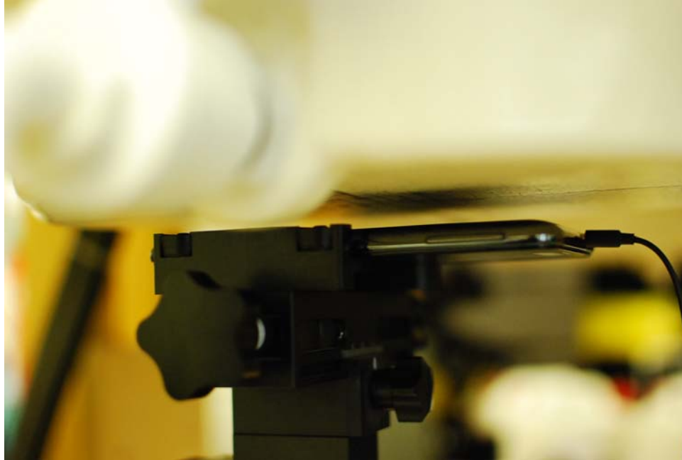
SAR Test Setup Photo 11: Body-Worn at 1.0 cm
