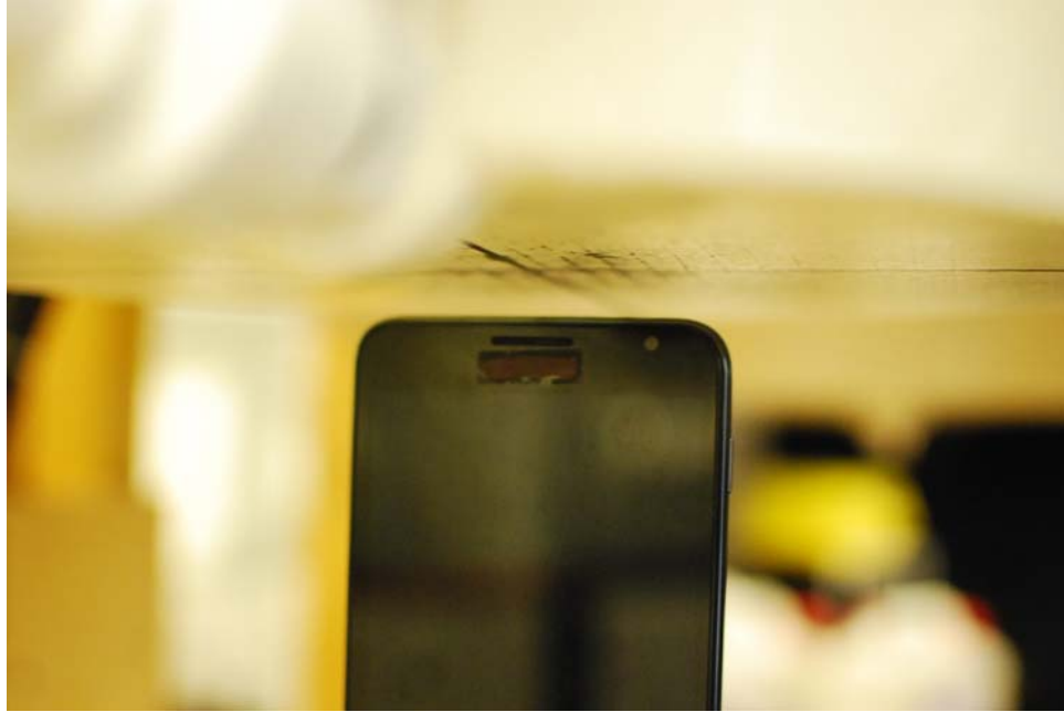
SAR Test Setup Photo 7: Top at 1.0 cm
