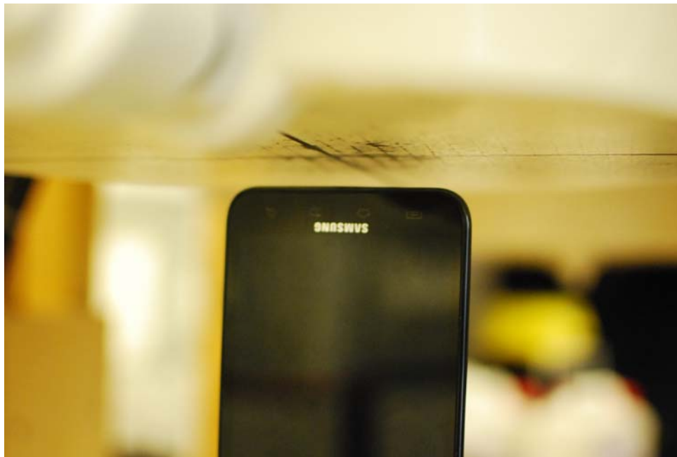
SAR Test Setup Photo 8: Bottom at 1.0 cm
