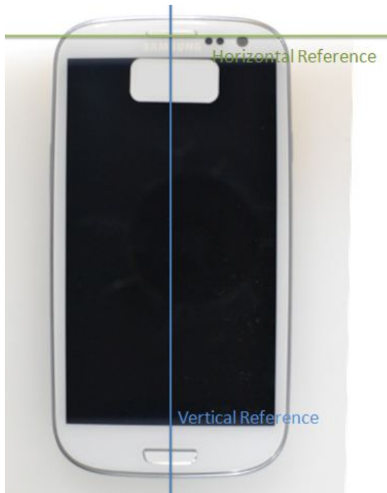
SAR Test Setup 11: DUT Horizontal and Vertical Reference Line
