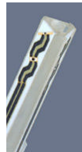
Figure 3.4 Probe Thick-Film Technique
