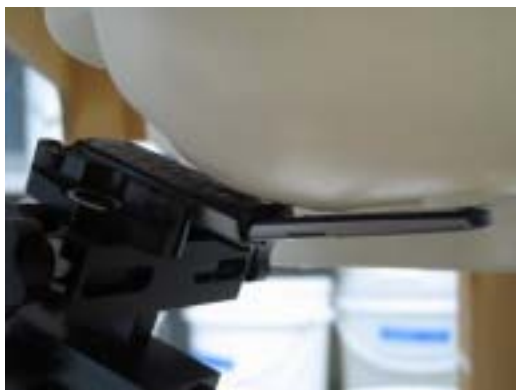
Figure 8.4 Left Head SAR Test Setup -- Cheek / Touch Position--
