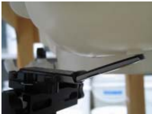
Figure 8.5 Left Head SAR Test Setup -- Ear/Tilt 15° Position--
