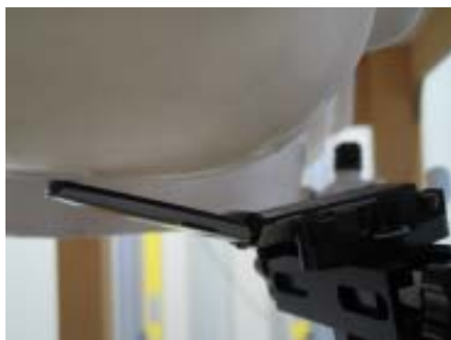
Figure 8.3 Right Head SAR Test Setup -- Ear/Tilt 15° Position--
