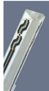
Figure 3.4 Probe Thick-Film Technique
