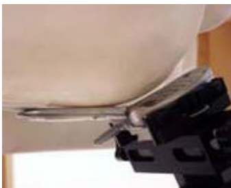
Figure 8.6 Right Head SAR Test Setup -- Cheek / Touch Position--
