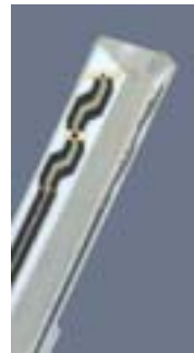
Figure 3.4 Probe Thick-Film Technique
