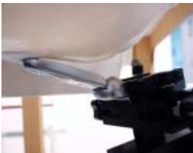
Figure 8.3 Right Head SAR Test Setup -- Ear/Tilt 15° Position--
