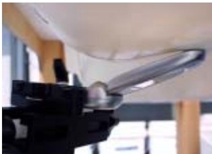
Figure 8.5 Left Head SAR Test Setup -- Ear/Tilt 15° Position--
