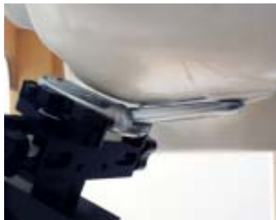
Figure 8.4 Left Head SAR Test Setup -- Cheek / Touch Position--
