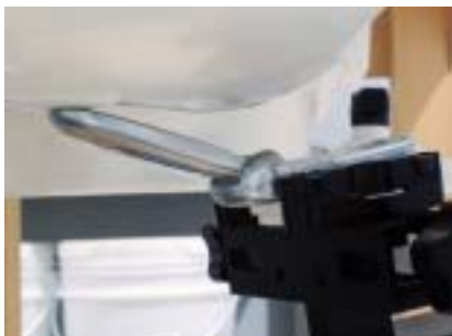
Figure 8.3 Right Head SAR Test Setup -- Ear/Tilt 15° Position--
