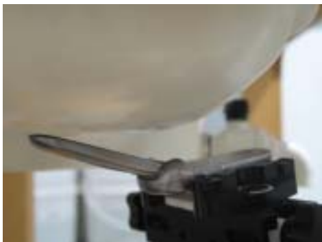
Figure 8.3 Right Head SAR Test Setup -- Ear/Tilt 15° Position--
