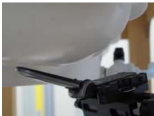
Figure 8.3 Right Head SAR Test Setup -- Ear/Tilt 15° Position--
