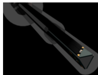
Figure 4-3 Triangular Probe Configuration
