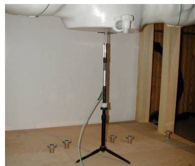
Figure 14-2 System Verification Setup Photo
