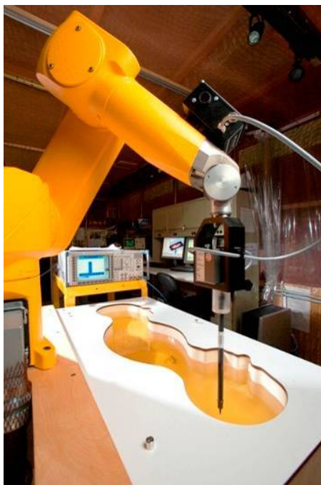
Figure 3-2 SAR Measurement System
