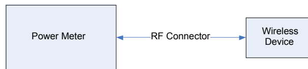
Figure 9-3 Power Measurement Setup
