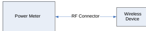
Figure 9-2 Power Measurement Setup
