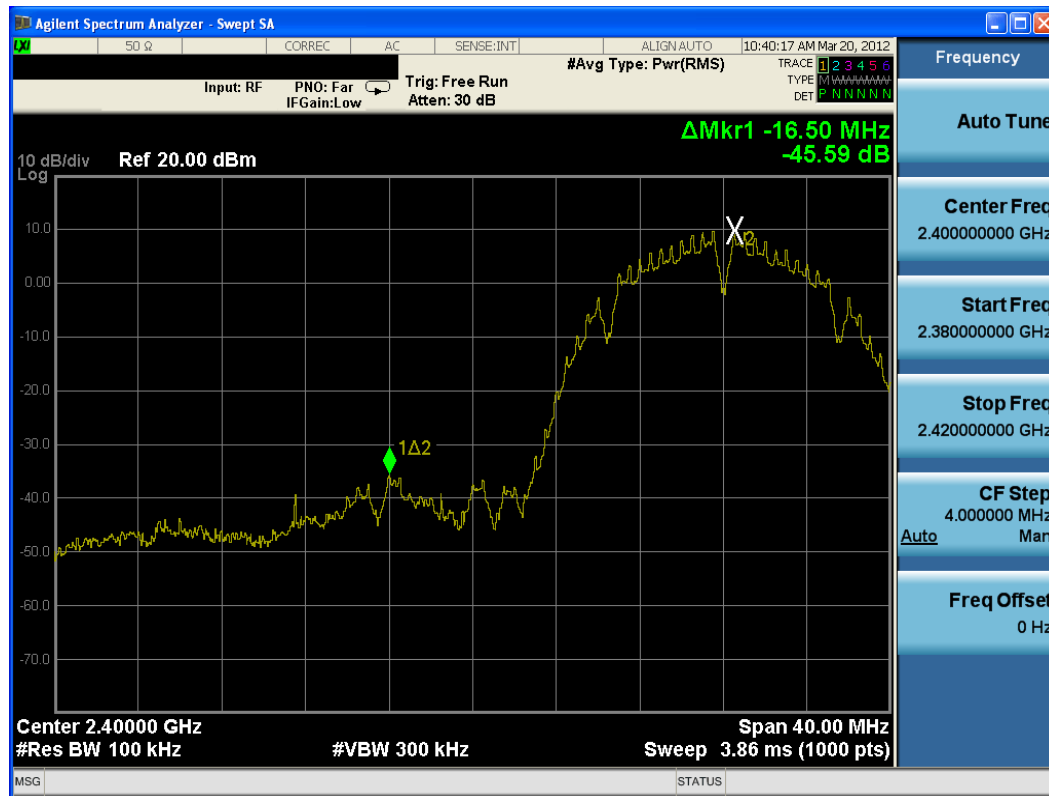
Plot 6-31. Band Edge Plot (802.11b – Ch. 1)
