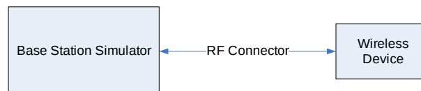
Figure 9-1 Power Measurement Setup
