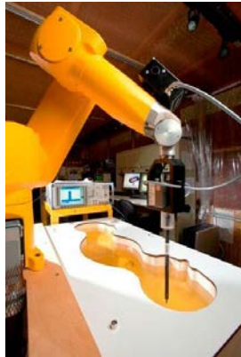
Figure 3-1 SAR Measurement System
