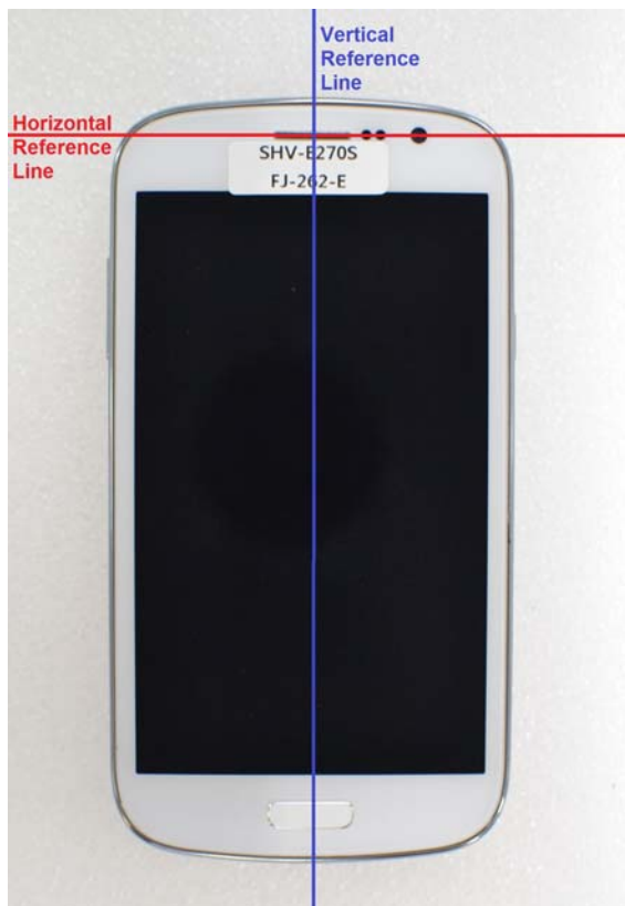
SAR Test Setup Photo 12: Vertical and Horizontal Reference Lines
