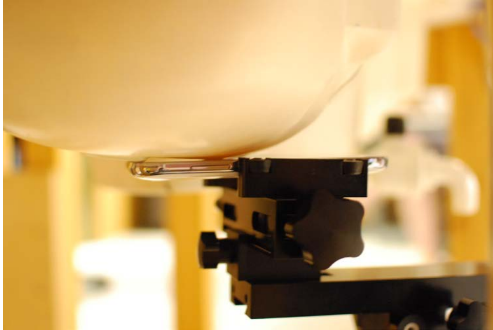
SAR Test Setup Photo 1 - Right Cheek Antenna Retracted
