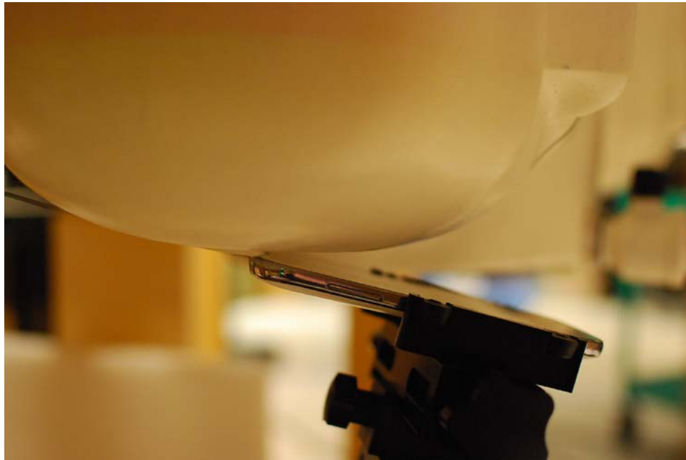
SAR Test Setup Photo 4 - Right Tilt Antenna Extended
