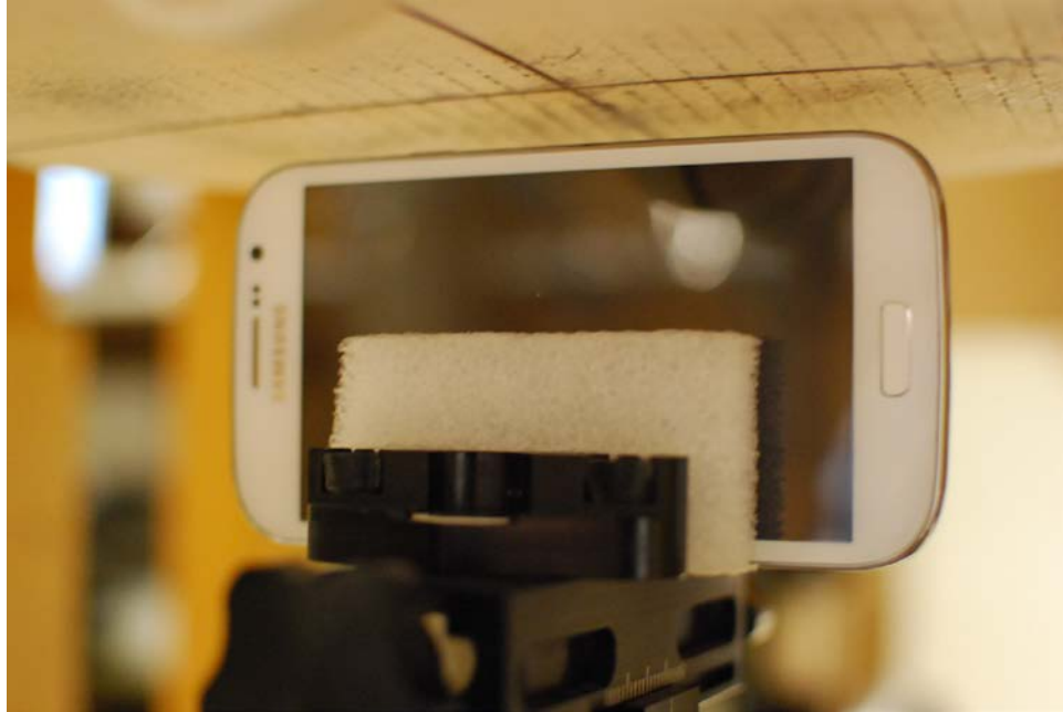
SAR Test Setup Photo 13 - Right Edge at 10 mm
