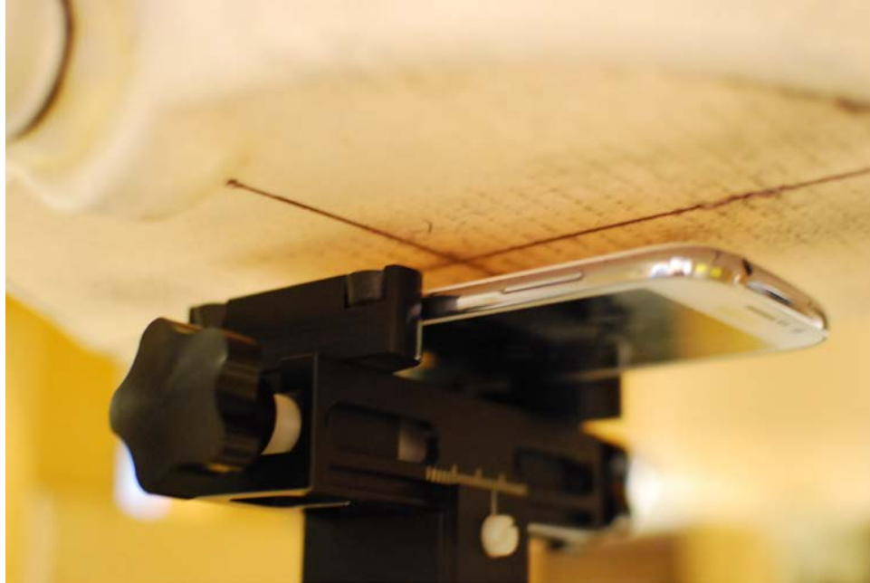
SAR Test Setup Photo 9 - Back Side at 10 mm
