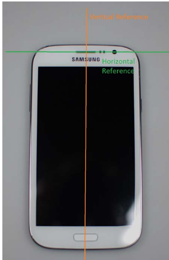
SAR Test Setup Photo 15 - Vertical and Horizontal Reference Lines
