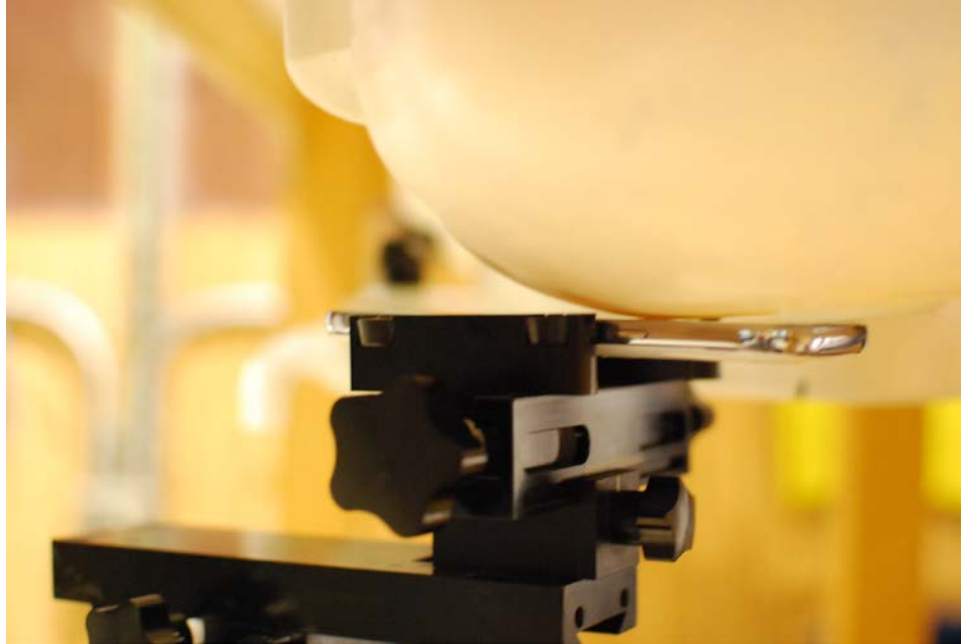
SAR Test Setup Photo 5 - Left Cheek Antenna Retracted
