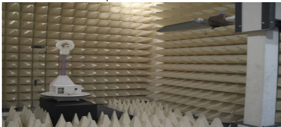
Figure2. Photograph of 3m Fully-Anechoic Chamber
