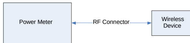
Figure 13-4 Power Measurement Setup
