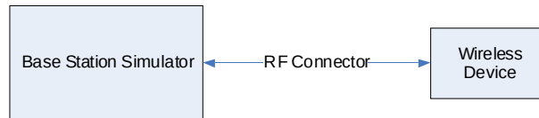
Figure 13-3 Power Measurement Setup
