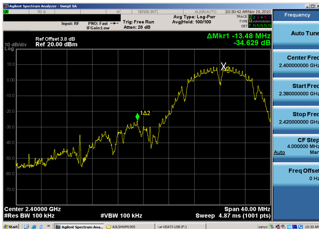
Plot 6-19. Band Edge Plot (802.11b – Ch. 1)
